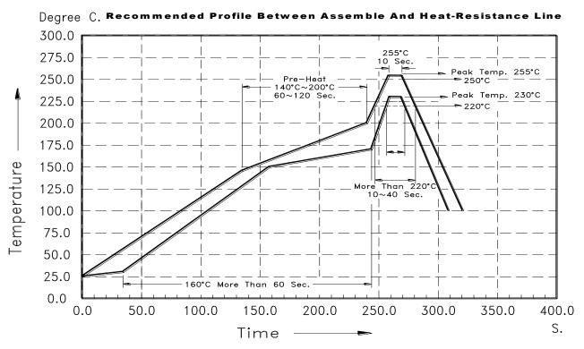
The Profile is available that must to use SnAg  $_{\left(x=3.3\sim3.8\right)}$  Cu  $_{\left(y=0.2\sim0.7\right)}$  solder paste
