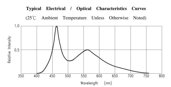
Fig.1 RELATIVE INTENSITY VS. WAVELENGTH
