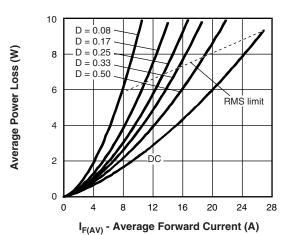
Fig. 6 - Forward Power Loss Characteristics
