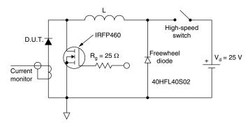
Fig. 8 - Unclamped Inductive Test Circuit
