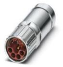
Cable connector, straight long, shielded: yes, Screw locking, M23, Number of positions: 4+4+4+PE, Type of contact: Male connector, Crimp connection, Cable diameter: 7.5 mm ... 9 mm
