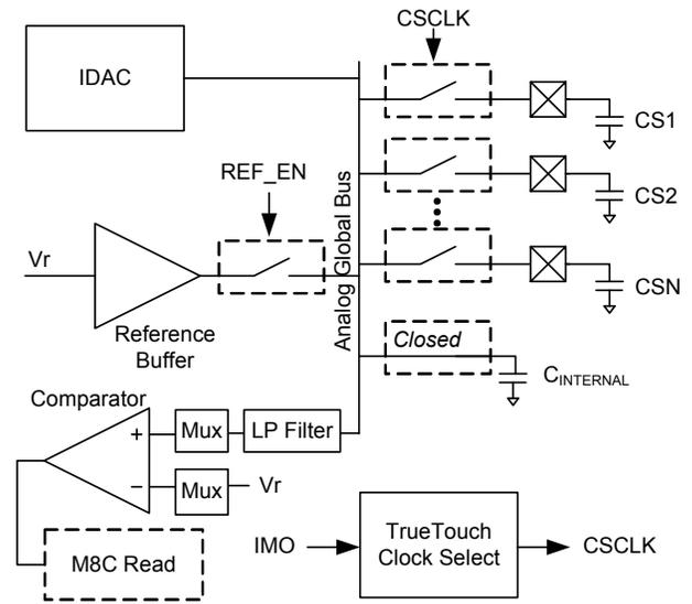
The reference bus is connected to the analog global line to initialize it to the Vr voltage (see Figure 11-7). After that, the reference buffer is disconnected and not used. The sense capacitance pin is now alternately grounded (see Figure 11-8) and connected to the analog global (see Figure 11-9). With the IDAC's current driving onto this net, the global net alternately charges and discharges a small amount.
