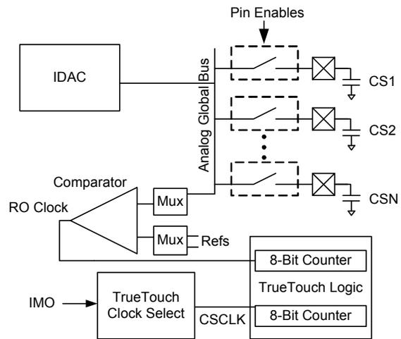
In the second RO method, the interval is set by a number of cycles of the RO using a 6-bit counter. During this interval, the IMO clocks a 16-bit counter and the final count gives a measure of capacitance. (See Figure 11-5.)
