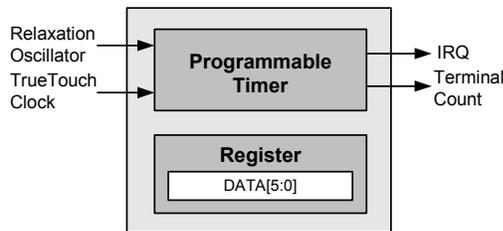
The timer's clock is either the 32 kHz clock (RLO) or the TrueTouch count clock, depending upon the value of the PXD\_EN bit in the CS\_CR2 register. See the [CS\\_CR2 Register on page 93](#) for details.
