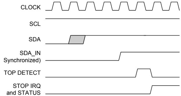
Figure 15-10 illustrates the timing for bus error interrupts. Bus Error status (and interrupt) occurs one cycle after the internal Start or Stop detect (two cycles after the filtered and synchronized SDA input transition).
