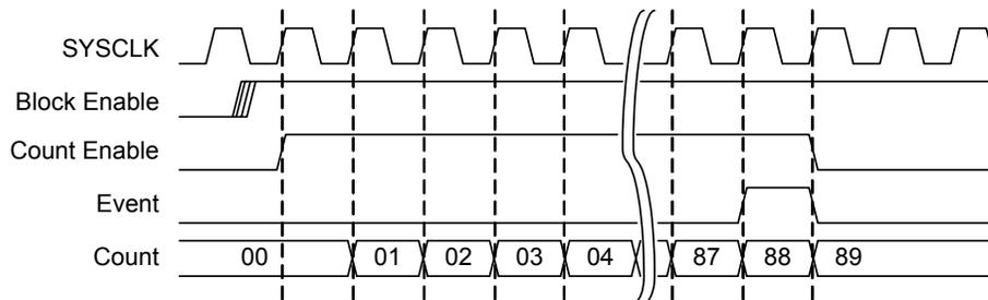
Figure 11-16. Pulse Width Frequency Timing (Mode = 01/10)
