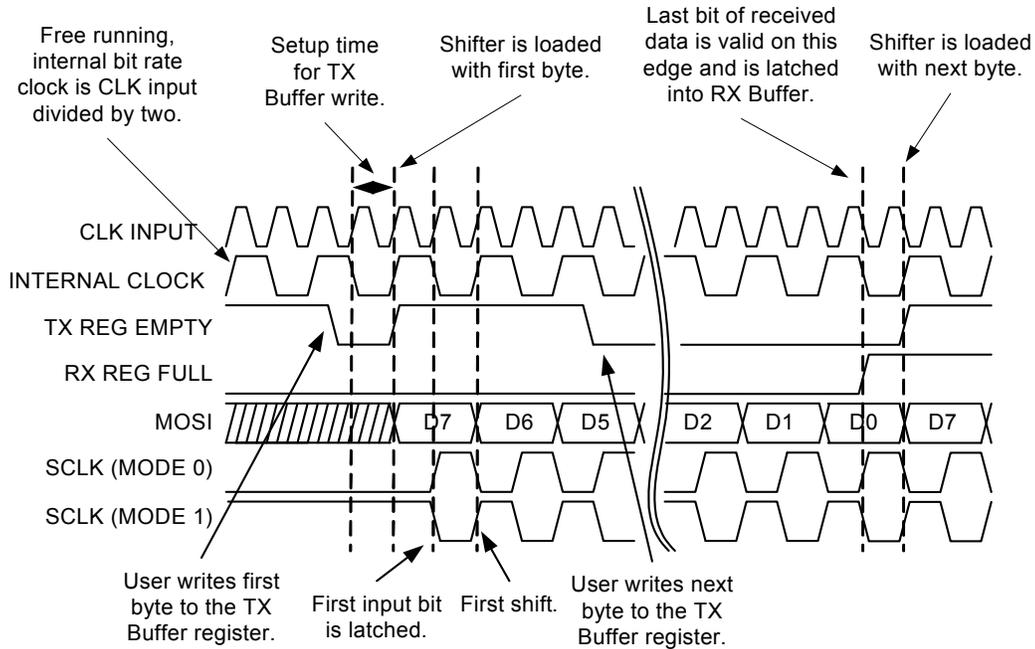
Figure 18-6. Typical SPIM Timing in Mode 2 and 3
