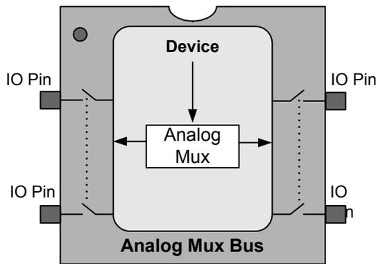
For each pin, the mux capability exists in parallel with the normal GPIO cell, shown in [Figure 12-2](#). Normally, the associated GPIO pin is put into a high impedance state for these applications, although there are cases where the GPIO cell is configured by the user to briefly drive pin initialization states as described ahead.
