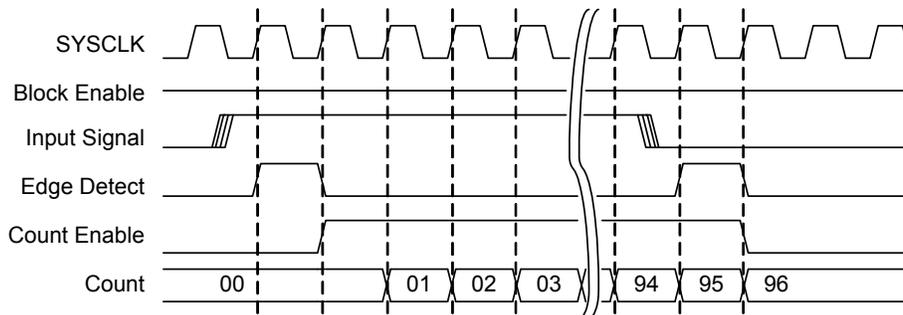
Figure 11-17. Continuous Timing (Mode = 11)
