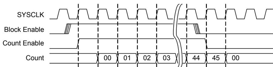
Figure 11-18. High Byte Counter Timing (RLO Clock Selected)
