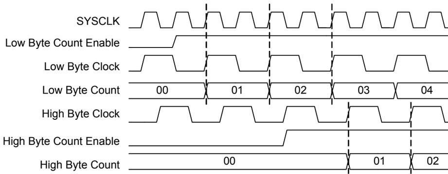
Figure 11-19. 6-Bit RLO Timer Operation
