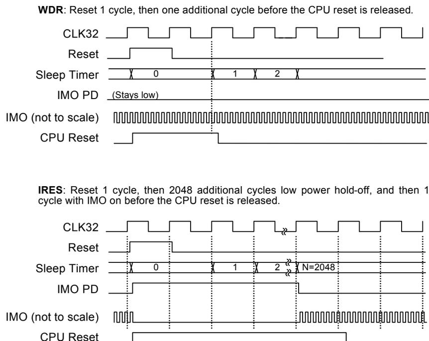
Figure 16-4. Key Signals During POR and XRES
