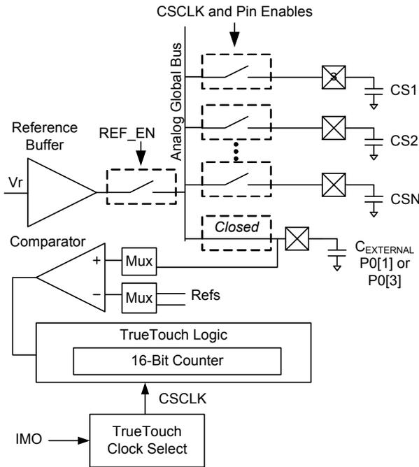
The initialization phase for negative CI (charge integration) is the same as for successive approximation (Figure 11-7). Following that, a two-phase sequence discharges the integration capacitor, as illustrated in Figure 11-11 and Figure 11-12.
