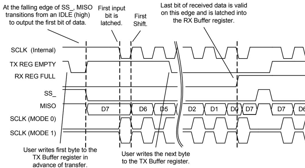
Figure 18-10. Typical SPIS Timing in Modes 2 and 3
