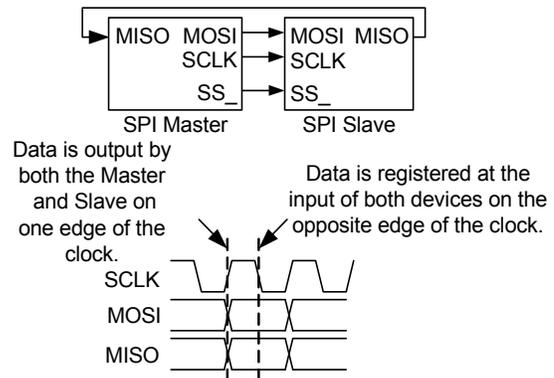
A device can be a master or slave. A master outputs clock and data to the **slave device** and inputs slave data. A slave device inputs clock and data from the master device and outputs data for input to the master. Together, the master and slave are essentially a circular Shift register, where the master generates the clocking and initiates data transfers.
