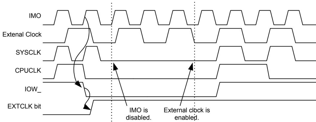
Figure 14-3. Switch from IMO to External Clock with the CPU Running with a CPU Clock Divider of One
