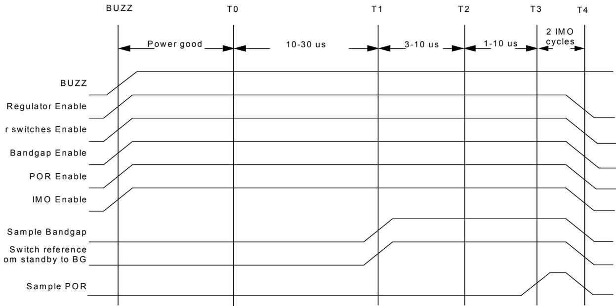
The buzz sequence after the Buzz signal comes. This is shown in [Figure 10-4, “Buzz Sequence Timing,” on page 80](#).
