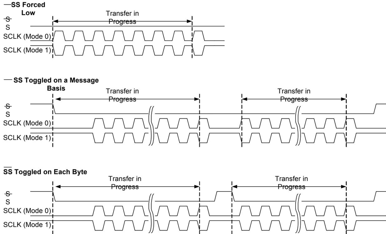
Figure 18-8. SPI Status Timing for Modes 2 and 3
