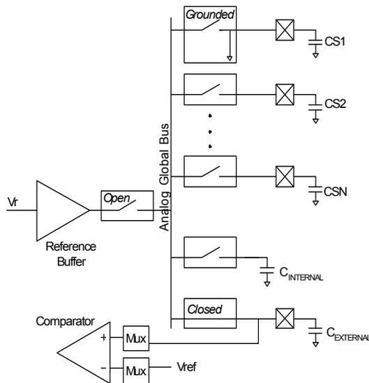
Figure 11-12. Negative Charge Integration Second Phase: Integrating Charge onto Integration Capacitor
