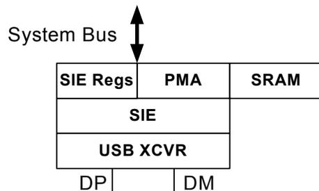
At the PSoC system level, the full-speed USB system resource interfaces to the rest of the PSoC by way of the M8C's register access instructions and to the outside world by way of the two USB pins. The SIE supports nine endpoints including a bidirectional control endpoint (endpoint 0) and eight uni-directional data endpoints (endpoints 1 to 8). The uni-directional data endpoints are individually configurable as either IN or OUT.
