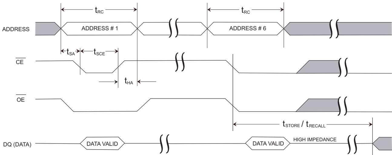
Figure 14.  $\overline{OE}$  Controlled Software STORE/RECALL Cycle [21]
