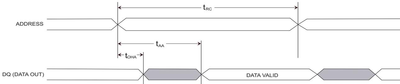
Figure 9. SRAM Read Cycle 2:  $\overline{CE}$  and  $\overline{OE}$  Controlled [10, 14]
