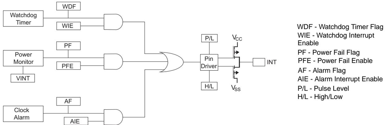
Figure 6. RTC Recommended Component Configuration
