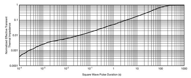
Normalized Thermal Transient Impedance, Junction-to-Ambient
