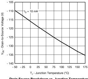
Drain Source Breakdown vs. Junction Temperature
