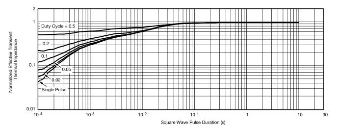
Normalized Thermal Transient Impedance, Junction-to-Case
